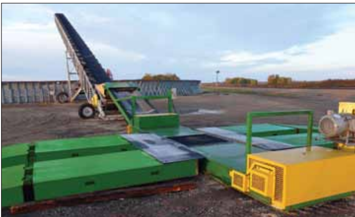
Tazz Corn Hog drive-over conveyor (lower right) delivers corn to a 15,000-bph Allatoona radial stacker. Photo courtesy of MaxYield Cooperative, West Bend, IA.
